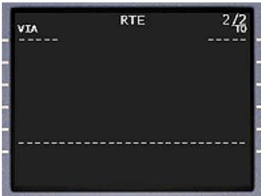
The RTE page 2/2 is where crewmembers manually enter the route of flight. This is accomplished by typing fix names individually into the scratch pad, then uploading them in order to the right LSKs.
