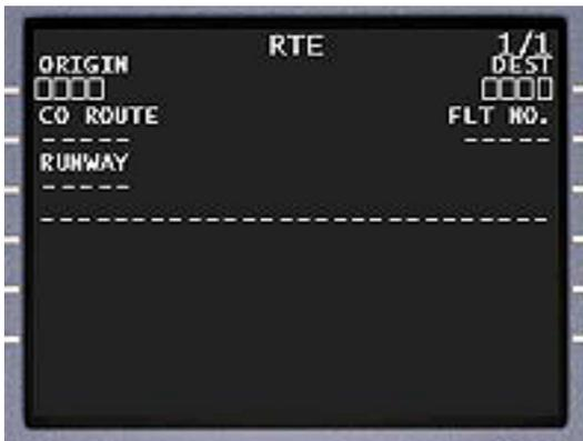
The RTE page is accessed either by pressing the RTE key on the FMC/CDU or
