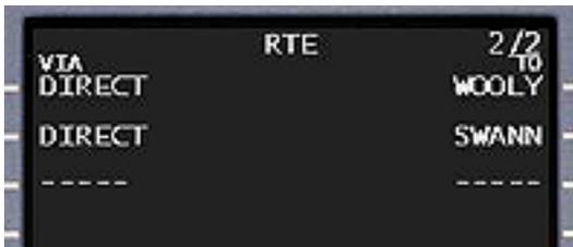
This would not be a correct according to our clearance as the cleared route of flight was to follow V214 from WOOLY to SWANN. (The BAL VOR is located between WOOLY and SWANN, but is not on a direct path between the two, so the route of flight turns slightly at BAL.)
