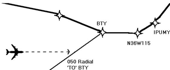
An Intercept Course entry is performed on the LEGS page. Enter the navigation fix that is desired into the scratch pad, the upselect
