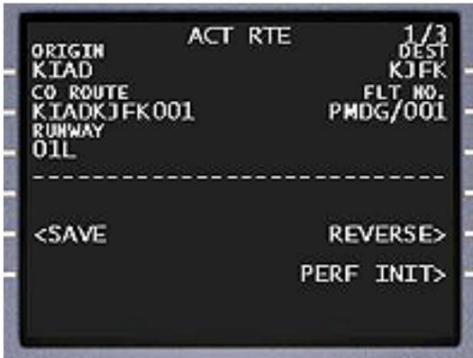
This will load the saved flight plan, and trigger the ACTIVATE> prompt so that crewmembers can confirm the route and EXEC it into active memory.
