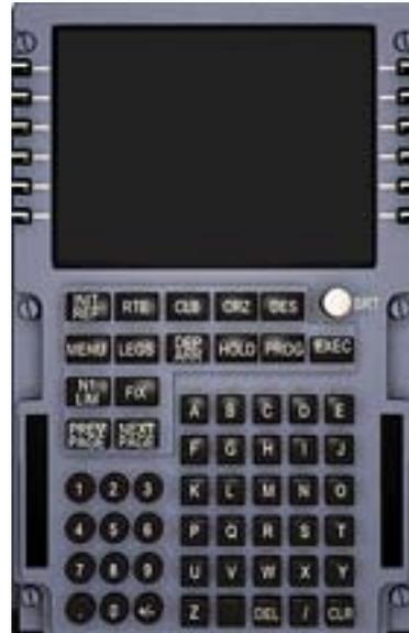
**FMC/CDU Display:** The MCDU display screen is comprised of 14 data lines capable of displaying 24 characters across in large or small font.
