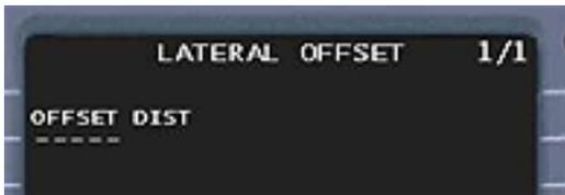
The desired lateral offset centerline can be entered by typing into the scratch pad and up-selecting to the 2L LSK.
