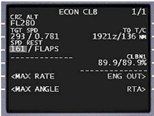
**CRZ ALT:** The cruise altitude that has been planned for the flight is displayed at 1L. The current cruise altitude is displayed if one has been selected and CLB is the active mode. If the current altitude is not displayed, 1L will contain prompt boxes which can be replaced by up-selecting the desired cruise altitude from the scratchpad.
