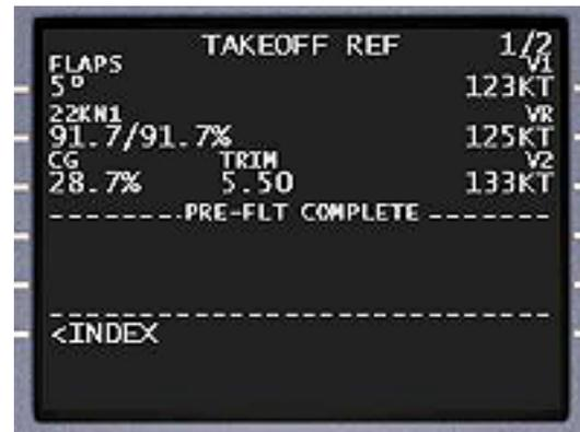
Flap Setting: The planned flap setting can be entered at line 1L. If an invalid takeoff flap setting is entered manually at 1L, an error message will be generated. The takeoff flap setting must be correct in order for the FMC to generate the correct takeoff speeds.
