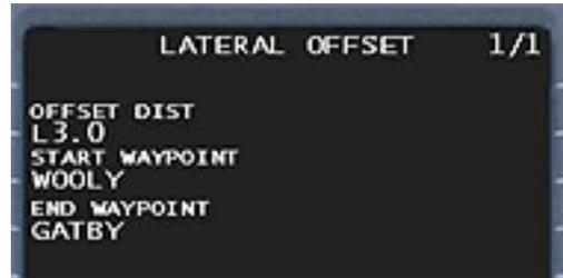
In this example case, the airplane will begin to fly 3.0 miles LEFT of the planned route of flight starting at WOOLY intersection. The aircraft will return to the normally planned centerline of the route at the GATBY intersection.
