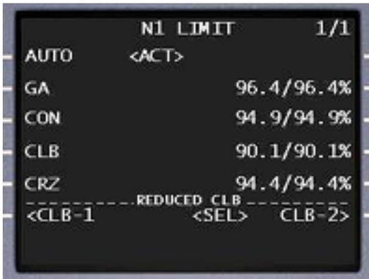
To select any of the various thrust limits available, simply press the associated LSK and the FMC/CDU will update the FMS to adjust the available thrust limit. Likewise, the CLB-1 and CLB-2 derated climb thrusts can be selected by pressing the associated LSKs near the bottom of the display.
