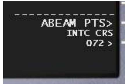
6R will show the current course to the desired waypoint. If a different intercept course is desired, it should be entered into the scratchpad, then up-selected to 6R by pressing the 6R key. This will instruct the FMS to intercept the desired course to the fix. The FMS will compute a great circle course between the current airplane location and the closest point of intercept to the desired course, and display that course on the ND as a dashed white line.
