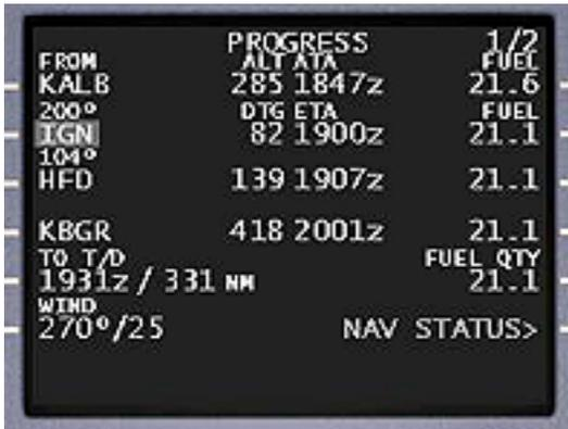
**FROM / ALT/ATA/FUEL:** The first line of the PROGRESS page display contains information related to the last flight plan fix that was over flown.
