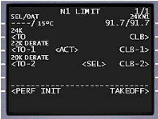
Available takeoff power derates are listed on the left side of the display while the climb power derates are available on the right side of the display.
