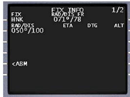
**NEXT PAGE/PREV PAGE Keys:** The NEXT PAGE and PREV PAGE keys are used in conjunction with MCDU displays which occupy more than one page on the MCDU display. Multiple page MCDU displays are indicated by the use of page numbering in the upper right hand corner of the MCDU display.
