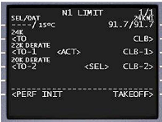
The N1 LIMIT page displays three takeoff thrust limit options at lines 2L through 4L. Lines 2R through 4R display climb thrust limit options. Additional information to help the crew obtain a clear picture of expected engine performance is also available from this page.
