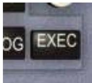
At any time the EXEC key is active, an <ERASE prompt will appear on the MCDU display in order to facilitate cancellation or deletion of a proposed action.
