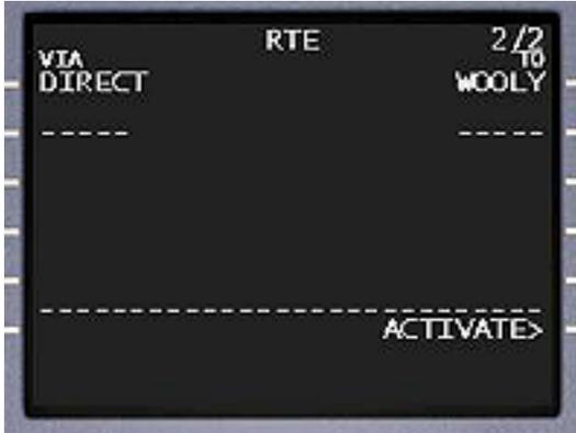
WOOLY is now displayed under the TO column on the RTE page 2/2. You will note that DIRECT is displayed under the VIA column, as the FMC/CDU assumes that it should fly DIRECT to any fix entered into the RTE page.
