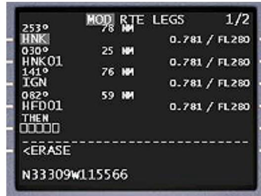
The entry is then up-selected to the desired line in the RTE LEGS display, where it will be condensed for display in the route, as shown below. The expanded entry can be redisplayed on the scratchpad by pressing the associated LSK.
