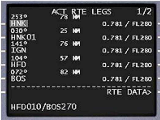
Once entered into the scratchpad, the PB/PB waypoint can be up-selected into the route by pressing desired LSK. The PB/PB waypoint is described in the route by the format XXXSS, where XXX represents the first three letters of the first waypoint's name, and SS is an FMC assigned sequence number.
