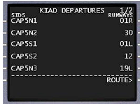
**SIDS:** The SIDS are listed on the left side of the display at 1L through 5L. A SID can be selected by pressing the associated LSK. Once a SID is selected, a <SEL> indicator will appear next to the associated SID to indicate that it has been selected by the crew.
