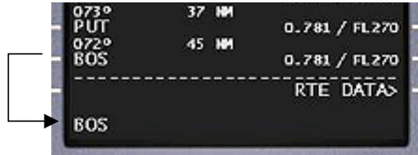
Then simply upselect the desired fix to the 1L LSK. This will cause the modified route to be displayed on the Navigation Display as a dashed white line, and will illuminate the EXEC key on the FMC/CDU to indicate that the route of flight change must be EXECUTED in order to take effect.
