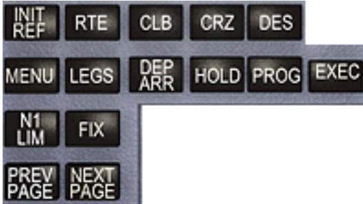
**MENU Key:** The MENU key provides access to the FMC and other aircraft sub-systems that use the FMC/CDU for input or control. When pressed, the MENU key brings up the following display screen on the FMC/CDU:
