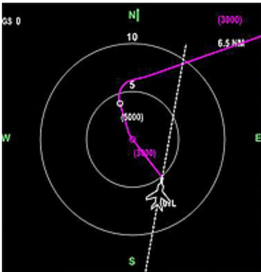
The fix that is currently the <CTR> cue in the FMC/CDU will be highlighted in white on the navigation display, and will be located at the center of the ND PLAN MODE display.
