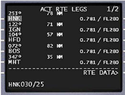
PBD bearing entries from 0 to 360 degrees and distance entries from 0 to 999 miles are valid
