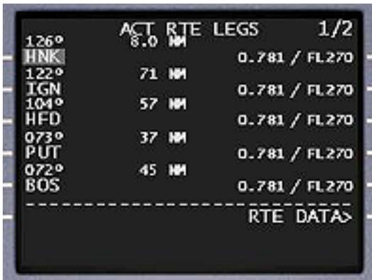
The simplest way to perform a DIRECT-TO change is to downselect or type the desired fix into the scratchpad:
