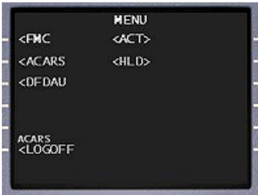
In the current version of the PMDG FMC, not all functions are active from this screen, as evidenced by the *grayed out* items in the menu. Currently only the FMC function is available by the FMC/CDU, but ACARS functionality is planned.
