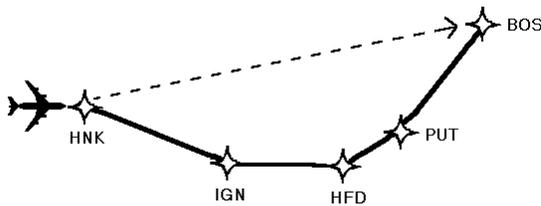
Direct-To routings are most easily accomplished by pressing the LEGS key on the FMC/CDU, and using the ACT RTE LEGS pages.
