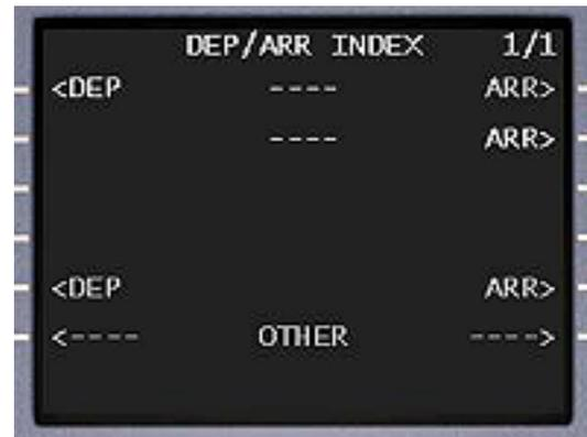
The DEP/ARR INDEX page allows the crew to select (using the appropriate LSKs) either the appropriate DEP procedure, or an ARR procedure for either of the two possible routes stored in the FMC
