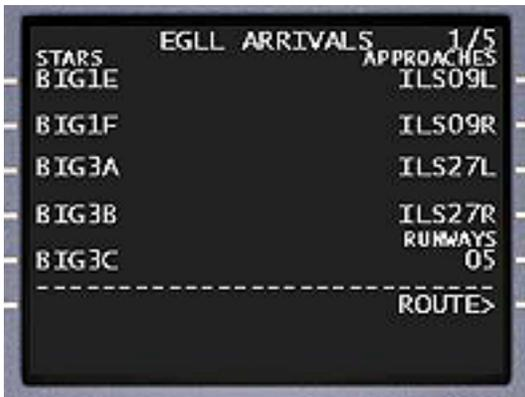
**Standard Terminal Arrival Route:** The STARs are listed on the left side of the display at 1L through 5L. A STAR can be selected by pressing the associated LSK. Once a STAR is selected, a <SEL> indicator will appear next to the associated STAR to indicate that it has been selected by the crew.
