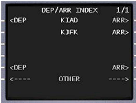
The 1L, 3L and 6L keys allow for selection of SID procedures stored in the FMC SID database. Keys 1R through 4R and 6R allow for selection of STAR procedures stored in the FMC STAR database. The center of the display shows the crew entered or COMPANY ROUTE entered arrival and departure ICAO airport codes.
