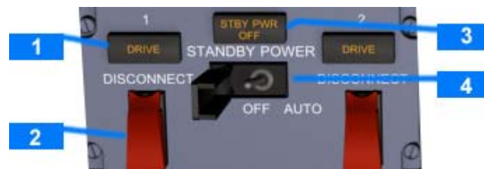
Forward Overhead Panel
