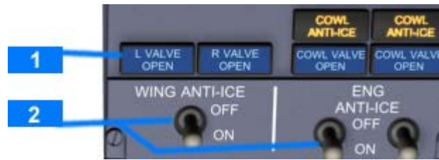
Forward Overhead Panel
