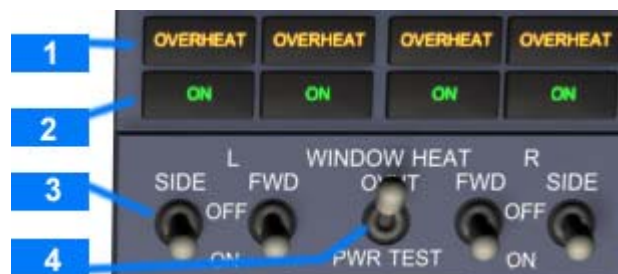
Forward Overhead Panel
