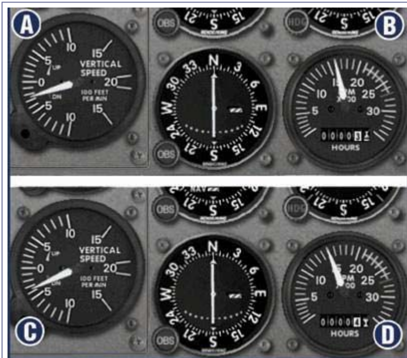
Figure 6-4 A-VSI and B-Tachometer with slightly more power. C-VSI and D-Tachometer with slightly less power.
