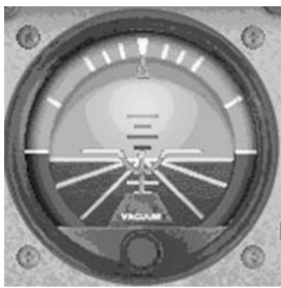
Figure 2-4 Mini-airplane rests almost on horizon bar in straight and level flight
